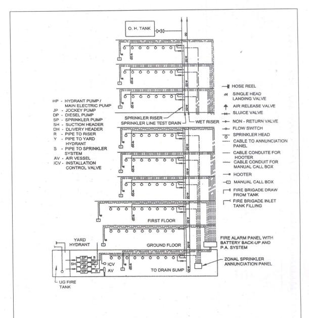
Fig 3 Typical Arrangement of Wet Riser and Total Sprinkler System of buildings Other than Apartment Exceeding 30 m in Height
